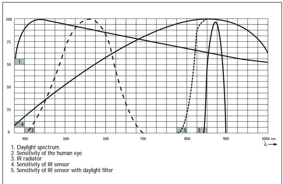
Fig 2.1 Infra-red radiation spectrum in relation to other spectra
