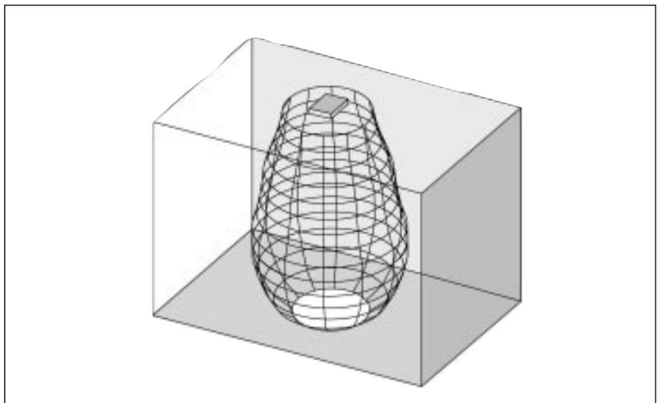
Fig 2.13 The radiator mounted perpendicular to the ceiling (i.e at  $90^\circ$  to the ceiling)
