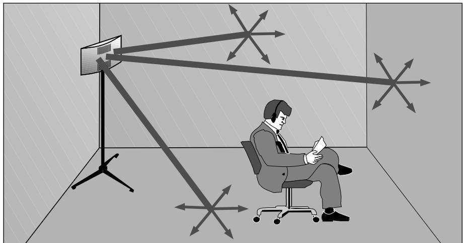
Fig 2.4 Combination of several reflected signals
