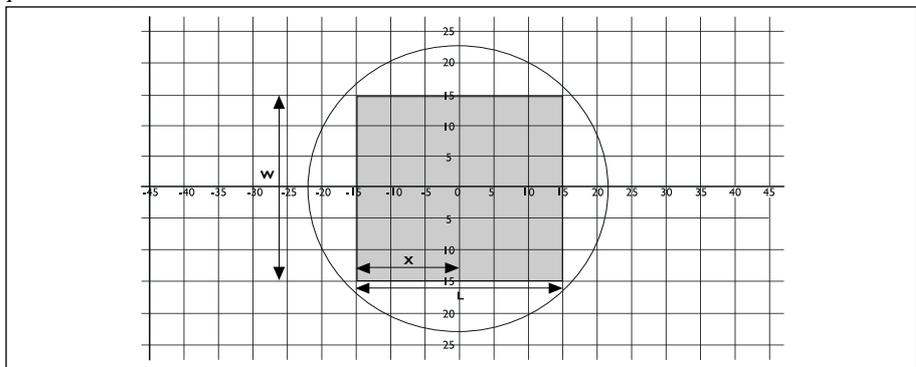
Fig 2.15 A typical radiator footprint for a mounting angle of 90°. X is negative because the radiator is actually mounted beyond the horizontal point at which the rectangular footprint starts.
