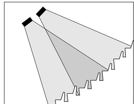
Fig 2.6 Radiator position (in cross-section) in a conference hall with very steep seating.
