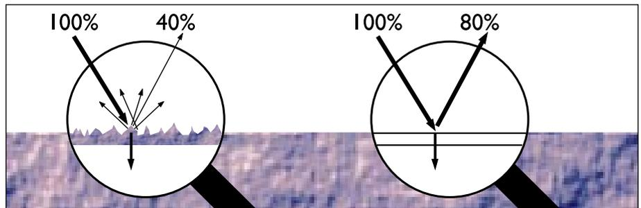
Fig 2.2 The texture of the material determines how much light is reflected and how much is absorbed
