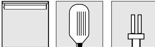
**Fluorescent lamps working at frequencies of up to 28 kHz** - energy-saving fluorescent lamps (without a dimming facility) which oscillate at 28 kHz, such as PL electronic lamps, may cause interference at up to 200 kHz (this interferes with channels 0 to 3). This interference can be overcome by using the upshift facility, which eliminates interference on these channels.
