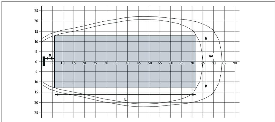
Fig 2.14 A typical radiator footprint for a mounting angle of 0°. The shaded rectangle shows the largest rectangular area where the signal-to-noise ratio is at least 40 dB(A). It is this area which is represented in the tables. The length (L), width (W) and horizontal point at which the rectangular footprint starts (X) are shown.
