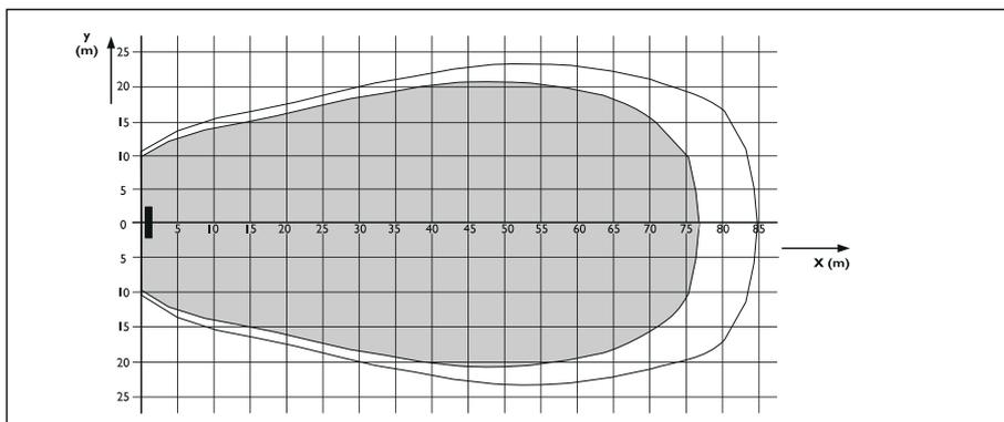
Fig 2.9 Example of an infra-red radiator footprint
