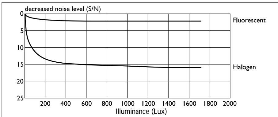
Fig 2.8 S/N ratio decrease when using fluorescent and halogen lighting
