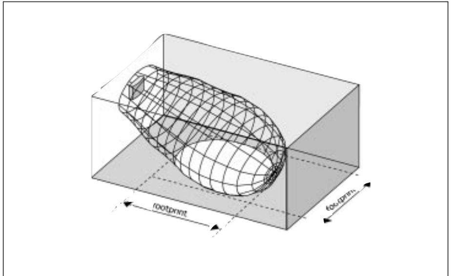
Fig 2.11 The radiator mounted at  $15^\circ$  to the ceiling
