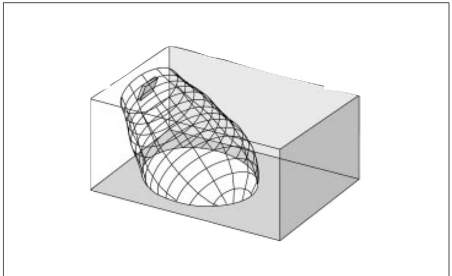
Fig 2.12 The radiator mounted at  $45^\circ$  to the ceiling
